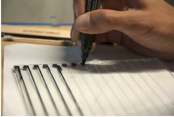
Figure 5: Customization of fabricated parts: a user increases the contrast of a transparent data scale by manually coloring previously engraved gridlines.
