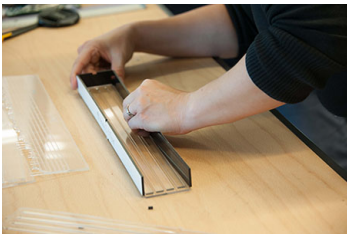
Figure 6: Assembly: parts cut by a laser cutter need to be put together to form a 3D visualization.
